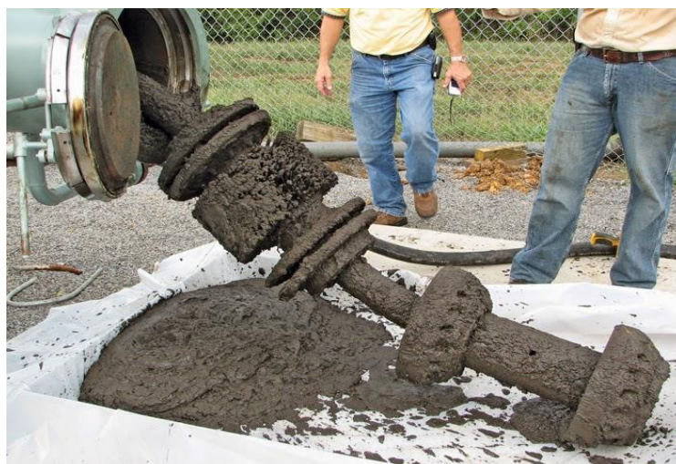
Figure 5: Result of pigging operation
